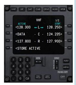
Figure E Tuning Control Panel
