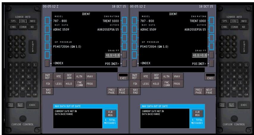
Figure D Lower MFD with Multifunction Keyboard (MFK). All MFDs are available as 2D Panels, but only the Lower has the MFK attached.
