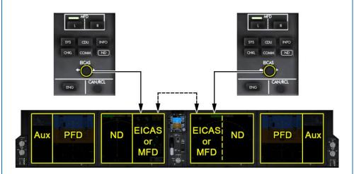
The EICAS transfer switches toggle the EICAS display between the Captain inboard DU and the First Officer inboard DU.
