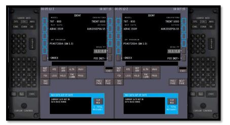
Figure D Lower MFD with Multifunction Keyboard (MFK). All MFDs are available as 2D Panels, but only the Lower has the MKF attached.
