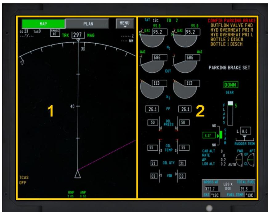
The inboard displays are capable of functioning as a Multifunction Display (MFD). As an MFD, it can operate as a Split Display or a Full ND Display. When it's operating as a Split Display (Shown above), there are 2 sides of the display as highlighted in the graphic above.
