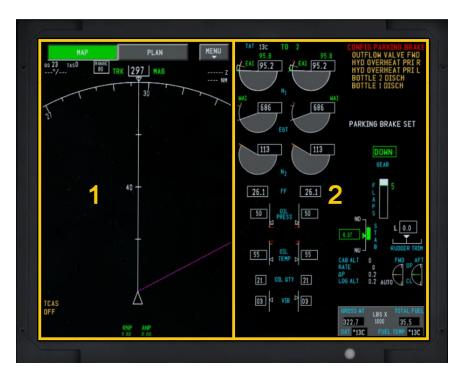
The inboard displays are capable of functioning as a Multifunction Display (MFD). As an MFD, it can operate as a Split Display or a Full ND Display. When it's operating as a Split Display (Shown above), there are 2 sides of the display as highlighted in the graphic above.
