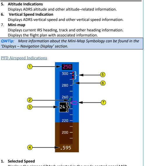
Displays the airspeed/Mach selected in the mode control panel MCP IAS/MACH window.
