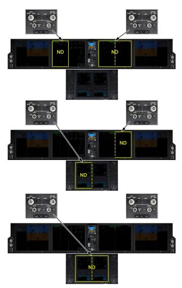
Each EFIS control panel controls the ND on the same side. If an ND is displayed on both MFD windows of the lower display unit, the 2 normal-display NDs combine to form a single full-display ND. The Captains EFIS control panel is used to control the full-display ND.
