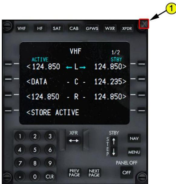
Once it's open, you can also close it using the (1) Close Switch on the top right corner of the panel.
