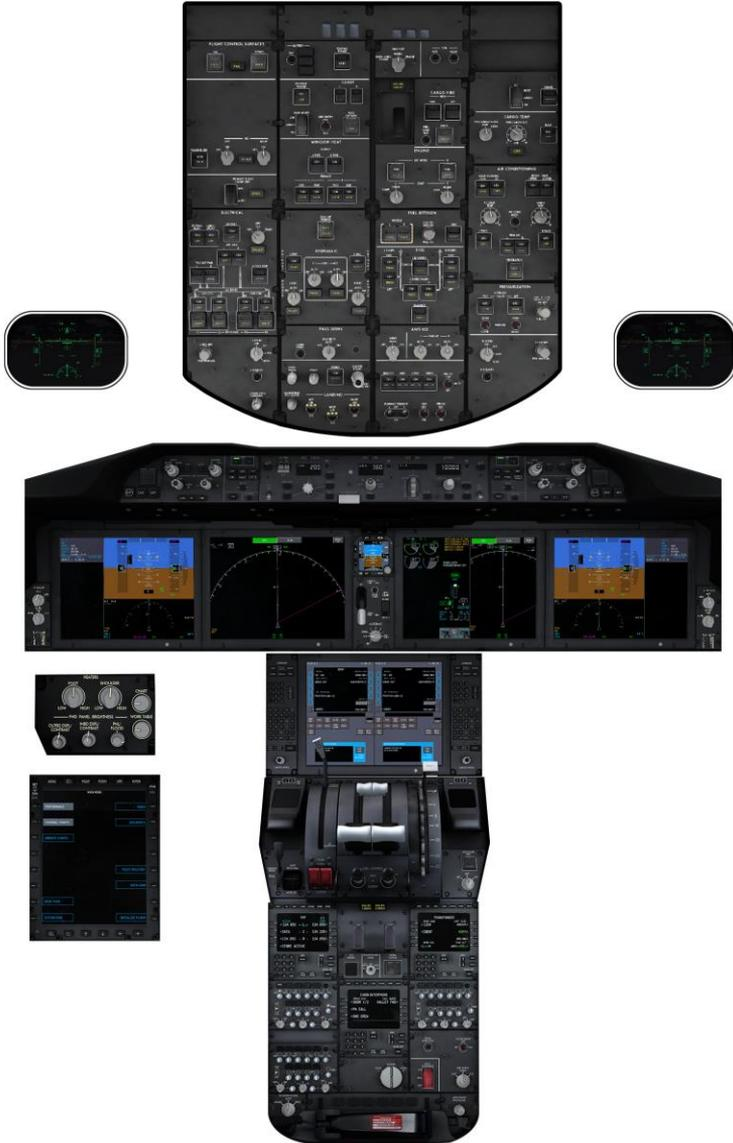
The overhead is sectioned into four columns, within each column are a different number of subpanels, grouping together the buttons, switches, knobs, and lights that represent the status and control of a particular system.
