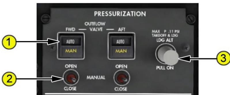
**1—OUTFLOW VALVE (FWD/AFT) Switches**
