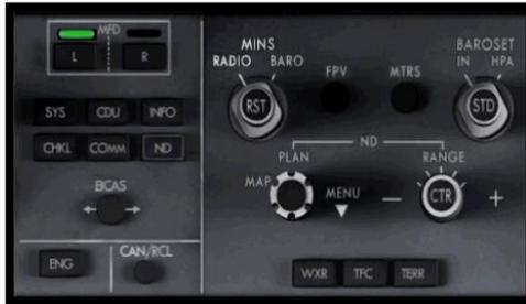
Figure F EFIS Control Panel
