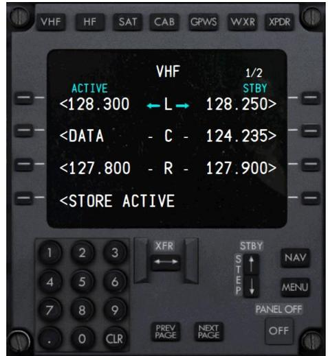
Figure E Tuning Control Panel
