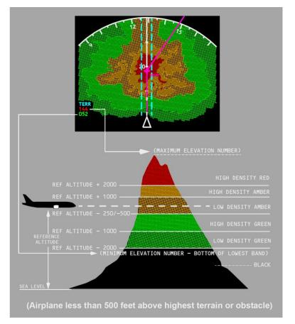
When a terrain alert occurs, the respective message is displayed on the ND. Terrain and weather radar cannot be simultaneously displayed on the same ND or mini-map, although, for example, a pilot can display weather on his ND, and terrain on his mini-map.
