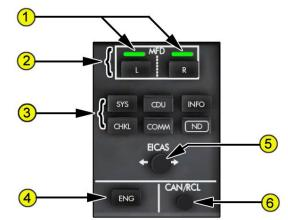
**1—Display Lights** Illuminates to show the MFD window the display select panel controls.
