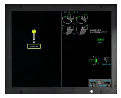
**1—Select MFD** If the number of instances requested for a display format exceeds the maximum available, SELECT MFD shows on the display
