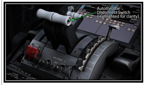
The autothrottle can also be disconnected manually by positioning both A/T ARM switches to OFF, or individually by positioning the left or right A/T ARM switch to OFF. Positioning one or both A/T ARM switches to OFF prevents activation of all autothrottle modes for the affected autothrottle.
