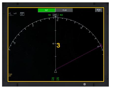
One Inboard Display can be selected to display a Full Navigation Display when the EICAS is occupying the inboard section of the opposite side Inboard DU.
