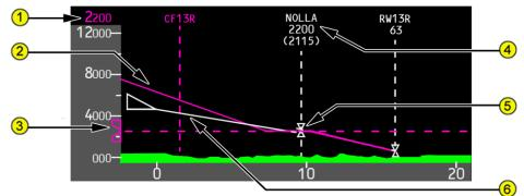
Displays the altitude set in the MCP altitude window.
