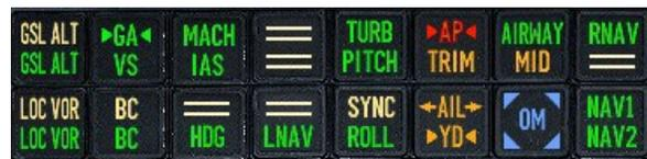
Figure XX: Flight Mode Annunciator Panel
