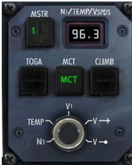
The Thrust Rating Panel (TRP) is a small panel to the right of the speedcard. It provides control over the maximum thrust settings for the engines for use with autothrottle.
