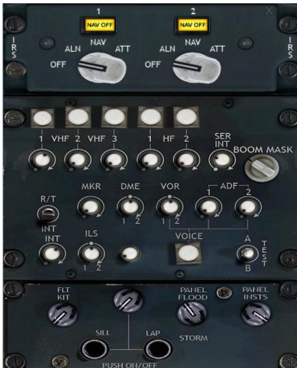
Avro RJ Audio Panel and IRS Controls ( Shift + 7 )
