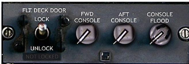
The Pedestal Lighting Controls can be found at the very aft portion of the pedestal
