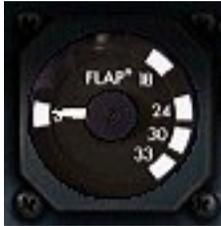
The flap indicator shows all of the flaps' positions. There are five indications on the flap indicator, each corresponding to the associated detent of the flaps lever on the throttle quadrant. The five detents are UP, 18, 24, 30 and 33. These indications have been placed around the outer edge of the flap indicator in such a way that they display the relative distances between the flap positions.
