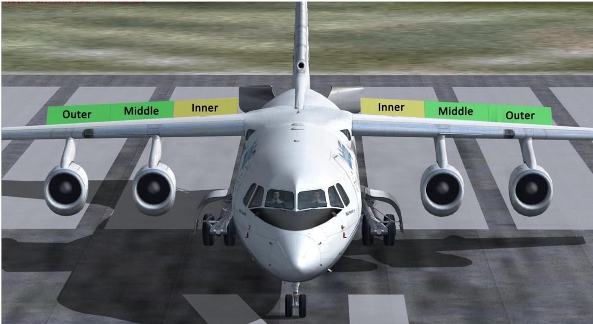
Figure 3: Lift spoilers: where, and by what hydraulic system (green or yellow)
