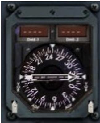
The Distance Bearing Indicator (DBI) is used for radio navigation. The instrument contains two LCD screens, which are distance indicators, and a compass with two dials, or bearing indicators. The two LCD screens display DME distance, while the bearing indicators display VOR or ADF bearings. The DME and VOR radios can be tuned via the VHF NAV controllers to the left and right of the MCP on the glare shield. The ADF radios can be tuned using the ADF box on the pedestal radio stack.
