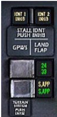
To the right of the gear position lever, there are several annunciator lights. The IDNT 1/2 and INHIB annunciators are related to the stall detection system. These are not simulated in this product.
