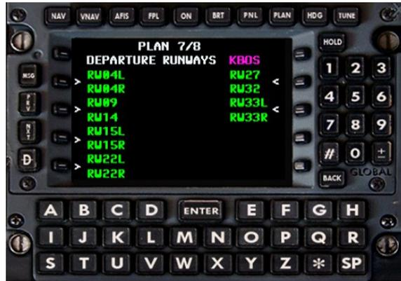
Plan page 7 is not present in the real GNS-XLS. It serves the purpose of being able to select a departure runway for airports without an available Standard Instrument Departure (SID). Since the real GNS-XLS in this case does not offer the capability to enter a runway, this page was added to enable the information to be entered for QWPAS announcements.
