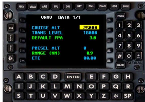
**CRUISE ALT:** Cruise altitude used by the FMS for TOC/TOD calculations. The value is pre-set when a flight plan is loaded into the FMS. This can be edited by pressing the LSK next to the cruise alt value (left side). The cruise alt will highlight in yellow. Then use the numeric keys to enter a new cruise altitude.
