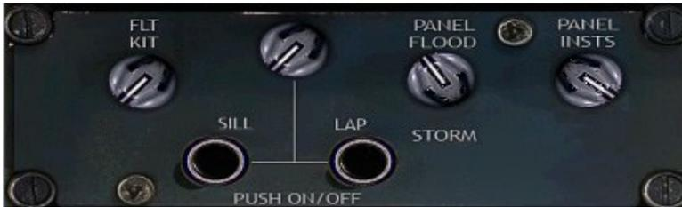
The main panel lighting controls can be found under the audio selector panel on the left side of the captain's seat and right side of the first officer's seat.
