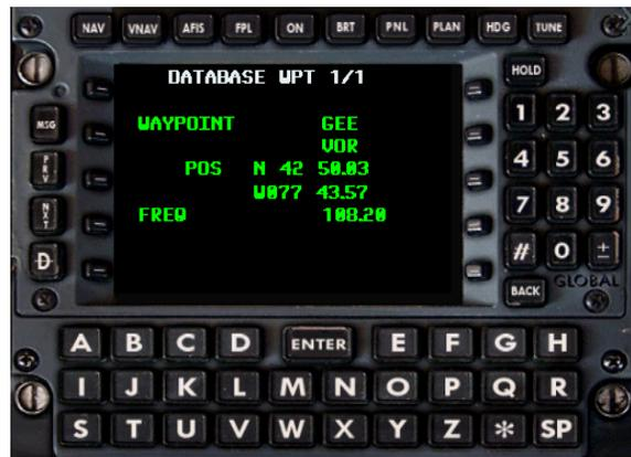
The database wpt page is displayed only when a new flight plan or direct to waypoint is entered to verify the entered identifier is indeed the navaid you wish to be inserted into the flight plan. By default the closest navaid with the same identifier to the aircraft's current position will be displayed.
