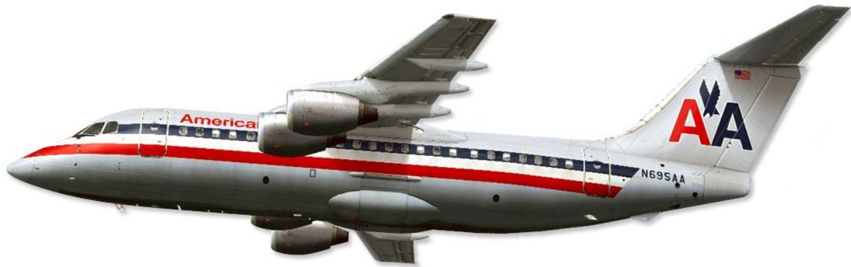
The BAe146-200 is essentially the same plane as the BAe146-100, only differing in length of the fuselage. The 200 was by no means meant as an upgrade of the original model in the way the Boeing 737-200 was an upgrade of the 100, for instance. Instead, the 100 and 200 were designed and built at the same time, the 200 being an extended version of the 100, capable of carrying a max of 112 passengers.
