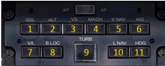
Figure 44: Autopilot engagement/disengagement controls
