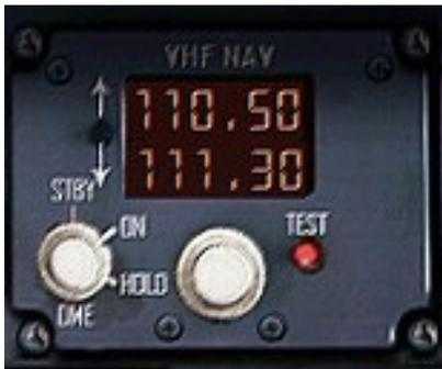
There are two VHF NAV panels on the Avro RJ / BAe146 series. One can be found to the left of the MCP, the other one to the right of the MCP panel. The left one controls the NAV 1 radio, the right one the NAV 2 radio. The Figure above shows the left NAV panel, which controls the NAV 1 radio.
