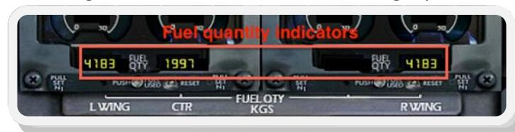
Figure 7: the fuel quantity gauges on the main instrument panel
