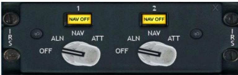
The IRS, or Inertial Reference System, is a system that gives situational awareness to the aircraft's systems. It uses inertia as reference to where it is and where it is going. It consists of an Inertial Reference Unit (IRU) and a Mode Select Unit (MSU). The MSU is the panel fitted on the First Officer's Audio panel. The IRU is a system not visible to the crew, but is controlled via the MSU. Together, they are called the IRS.
