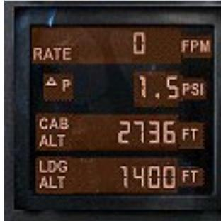
The first line shows the current cabin rate in feet per minute (FPM)
