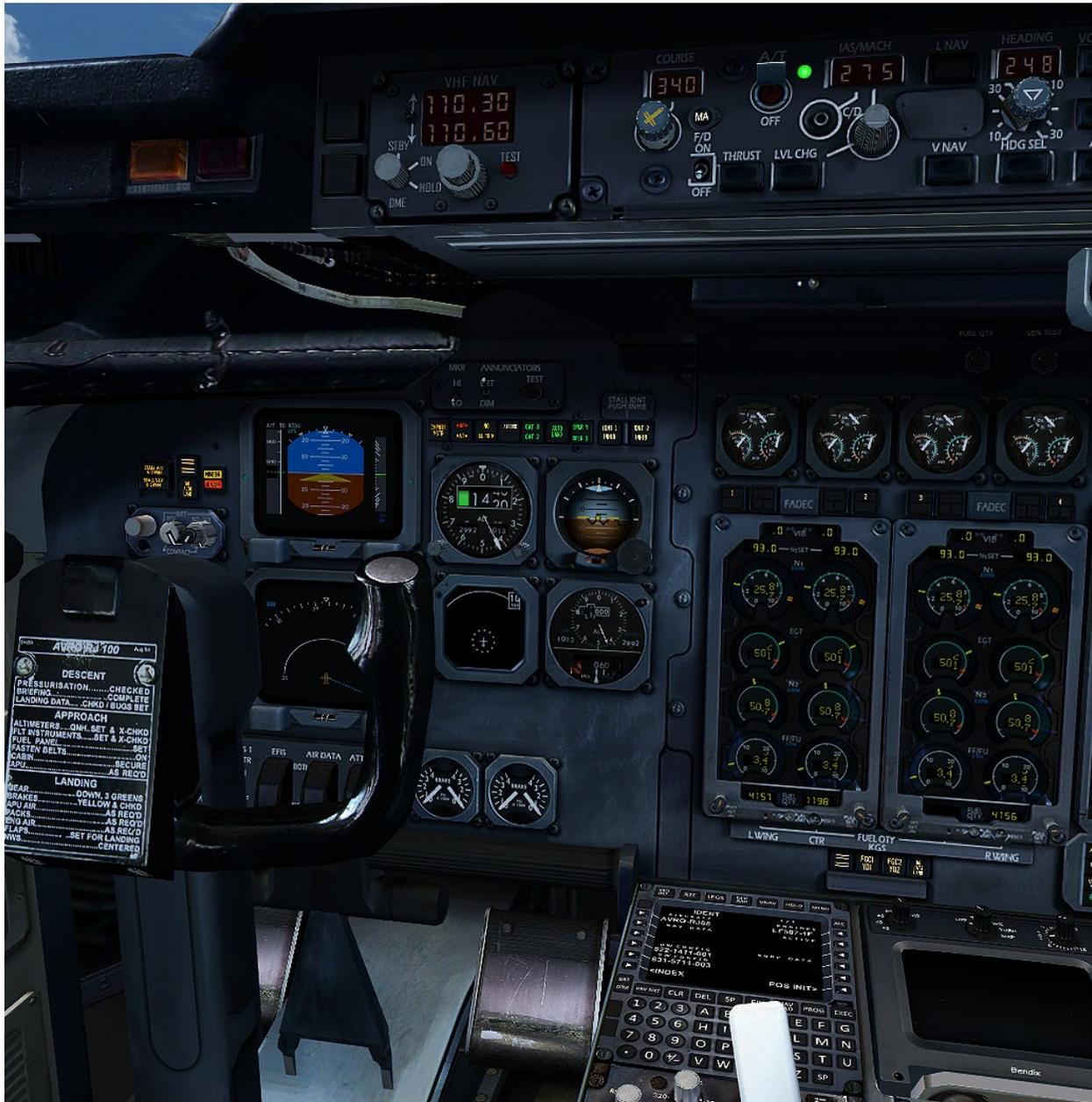
The Main Instrument Panel in the Virtual Cockpit
