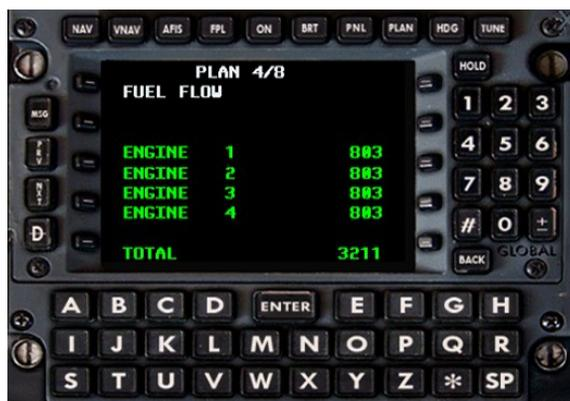
Individual engine fuel flow and total fuel flow.
