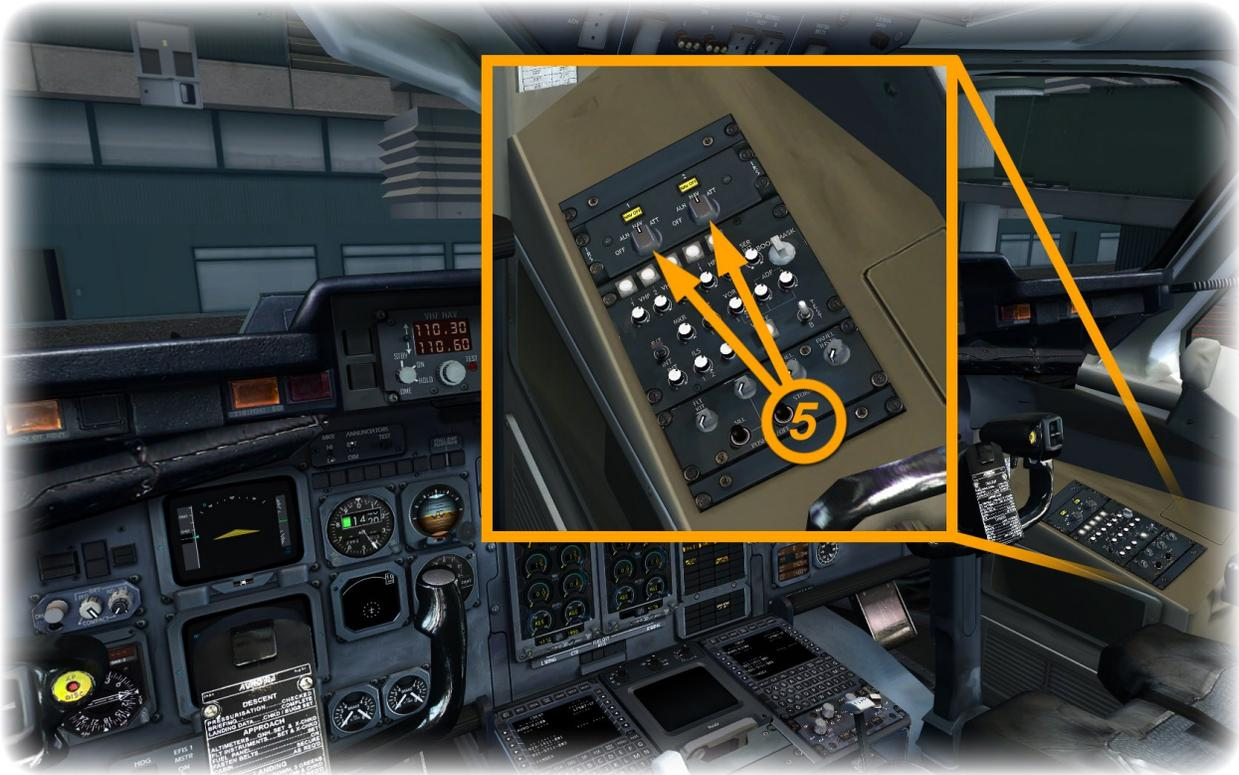
The Inertial Reference System (IRS) tells us where our plane currently is. As long as this system is not active, you won't see an artificial horizon on the Primary Flight Display as well as no navigation information on the Navigation Display.
