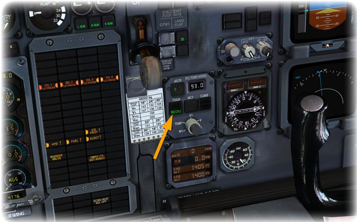
Now right-click on the outer ring to switch to the TEMP mode. This let's you set your Outside Air Temperature. The temperature is automatically preset to the current temperature. You can manually adjust the temperature if you wish.
