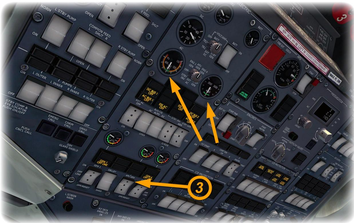
First move the APU GEN switch from OFF/RESET to OFFLINE by right-clicking it. This connects the generator drive to the APU.
