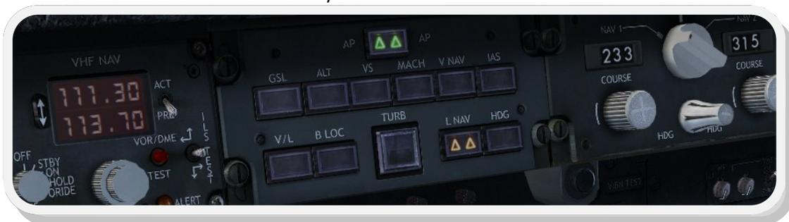
To slow down the plane it is suggested to change to VS or PITCH mode. The first holds the vertical speed at the time of engagement and allows you to decelerate while holding vertical speed. The latter is selected by de-selecting any other vertical mode and allows you to adjust your pitch by means of the small PITCH knob on the autopilot control panel (on the pedestal). It is labeled with 'UP'/'DN'. Slow down to be at approximately 190kts when passing 'TRAVA'.
