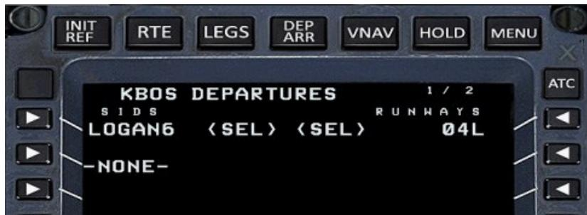
Return to the RTE page. You will see LOGAN6 inserted as an airway to the last waypoint of the SID. In this case this is HD036.
