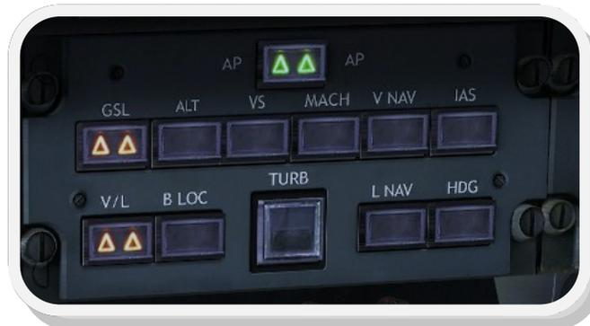
With the glideslope signal alive, select the gear down when you are 1.5 dots below the glideslope and select Flaps to 24° at 0.5 dots.
