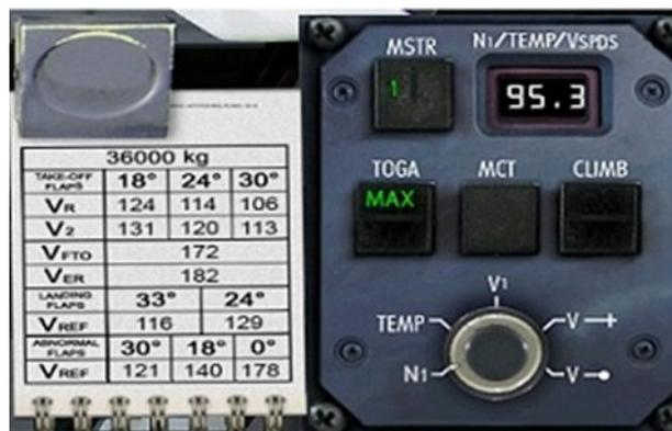
Flex is a reduced thrust takeoff. As Max is harder on engine life it is better to takeoff with less thrust if weight and conditions permit. Once again, flex data is runway and weight specific and therefore impossible for us so compute. BUT we can use a little bit of logic in our choice. If we are departing a 10,000 foot runway in flat country we can take a big reduction.
