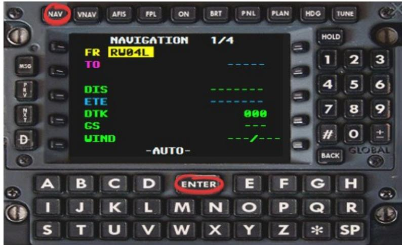
The first waypoint of the SID (HD036) will automatically show up in the TO field. Confirm this again by pressing ENTER.
