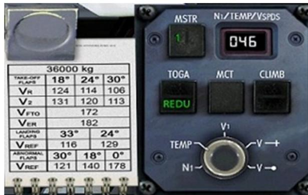
It is important to note when departing with a Flex temp that climb N1 will be reduced as well if we select NORM climb after takeoff. This can limit climb performance at high altitude. Therefore if you have a reduction you may want to remove the temperature set on the TRP at higher altitudes when the rate of climb falls below 1000 feet per minute.
