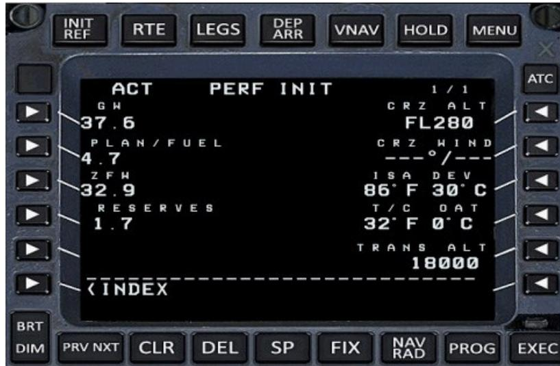
Next press the VNAV key. Enter a CLB speed of 270/.70M. This will vary depending on company policy or other factors such as headwind/tailwind. Generally a climb speed of 270-280kts transition to climb Mach of .65-.70 is good:
