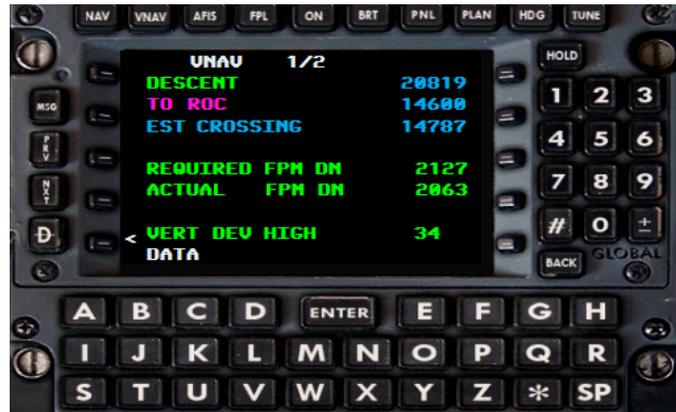
Select the **DESCent** mode on the TMS and observe if any arrows light up and signal the need for more thrust. If this is the case, you have fallen below the minimum N2 required for the engines to produce enough bleed air for anti-ice and air conditioning needs. Gently advance your throttles and wait for a reaction of the engine until the arrows extinguish. Use the airbrake if the required rate of descent cannot be reached.
