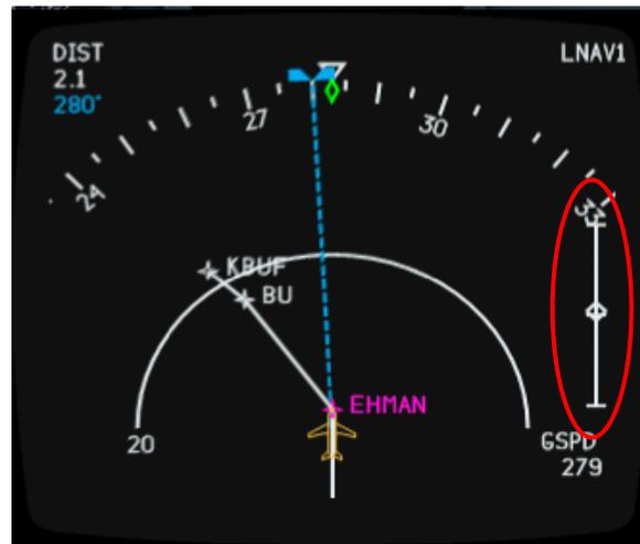
If the VDI does not show, make sure your Primary Course Selector on the EHSI control panel below the FMS is set to LNAV.
