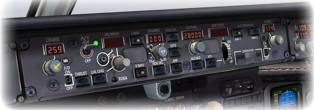
An important altitude during your climb is the 10,000ft mark. If you're flying in VNAV, the plane will automatically lower the nose and accelerate to the CLB speed programmed in the FMS. Below 10,000ft it will adhere to the 250kts restriction.
