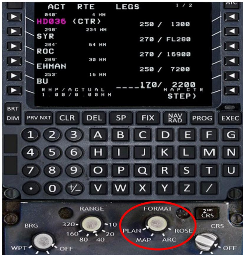
Should you see a route discontinuity, select the waypoint after it (here: BU) and insert it into the line that contains the discontinuity. Always press EXEC after any changes.
