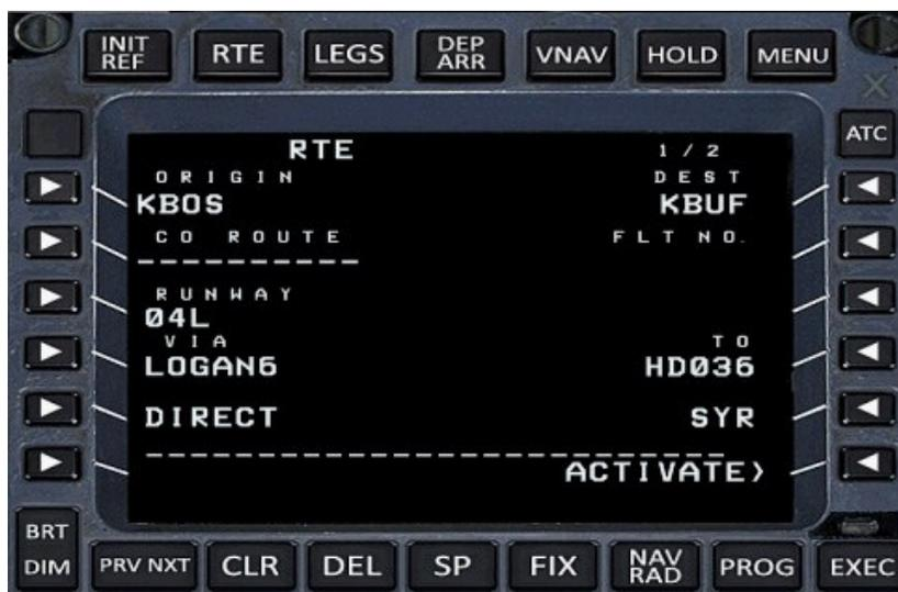
We have reached the end of the page. In the upper right corner of the screen you might have noticed that the page display changed from 1/1 to 1/2. You can now select between the pages via the PRV / NXT key in the lower left corner of the figure above.
