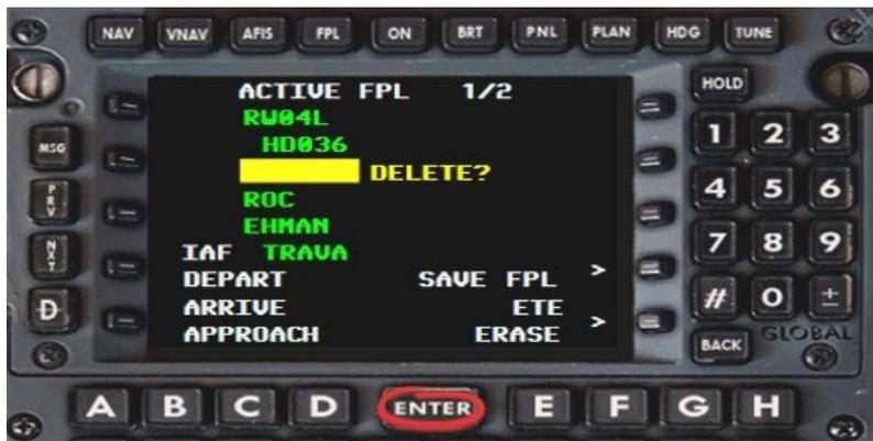
All waypoints of the route are inserted. Now we have to set up the vertical profile. For this, press the VNAV button in the upper row of buttons. The VNAV page will open. In order to insert the desired cruise altitude, press LSK 5L and ENTER.
