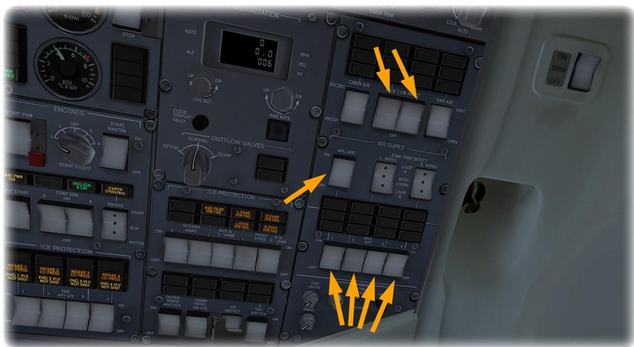
To avoid engine surge, your engine Anti-Ice system must be switched on. Should you miss this step, the Avro has an automatic system that switches on the Engine Anti-Ice system should an engine start be initiated without Engine Anti-Ice selected on.
