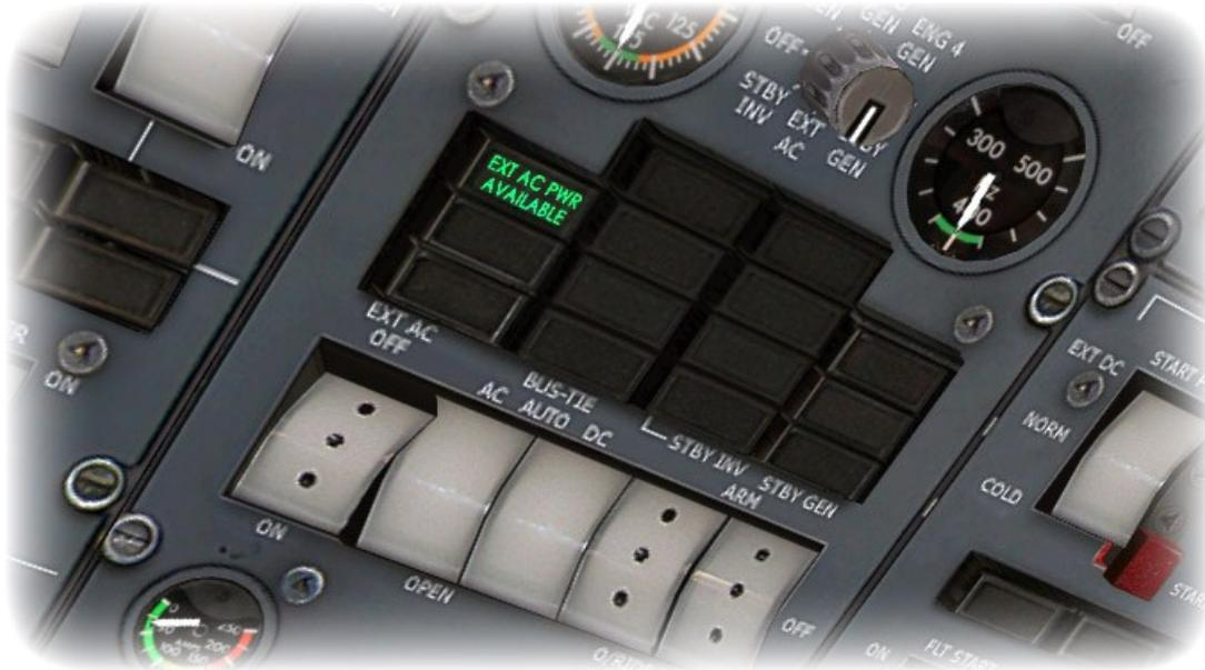
Now put the ENG GEN1 and ENG GEN4 switches to OFF/RESET. The switches are located right below the EXT AC switch.
