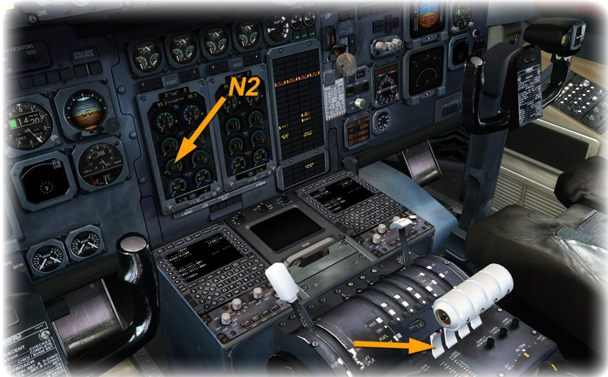
Monitor your primary engine display. At about 10% N2, right-click the fuel-cutoff switch on the thrust lever of the engine you're starting. This will move the thrust lever into the IDLE detent and give your engine fuel. You will see the ignition at about 20% N2.
