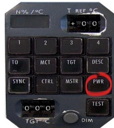
Select your current Outside Air Temperature in the 'T REF' thumbwheel window in the upper right corner of the control unit. Now click the 'TO' button. A green triangle will illuminate. The reference N1 value for your take-off will be displayed in the LED window. As soon as your thrust levers are within range of this reference N1, the TMS will try to achieve it by adjusting the actuators.
