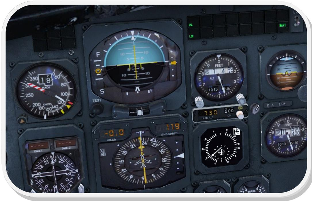
The BAe146 is not equipped with an Autoland function. Thus, when passing the decision height or a minimum of 160 feet radio altitude, disconnect the autopilot and commence a manual landing.
