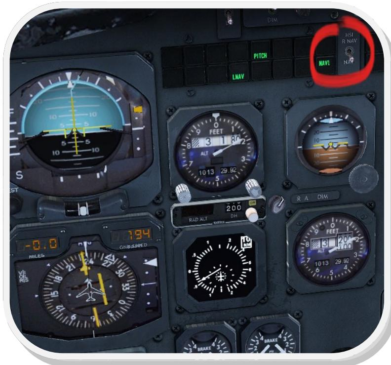
Arm the V/L and GSL autopilot modes, so that the plane can capture the localizer and glideslope signal.
