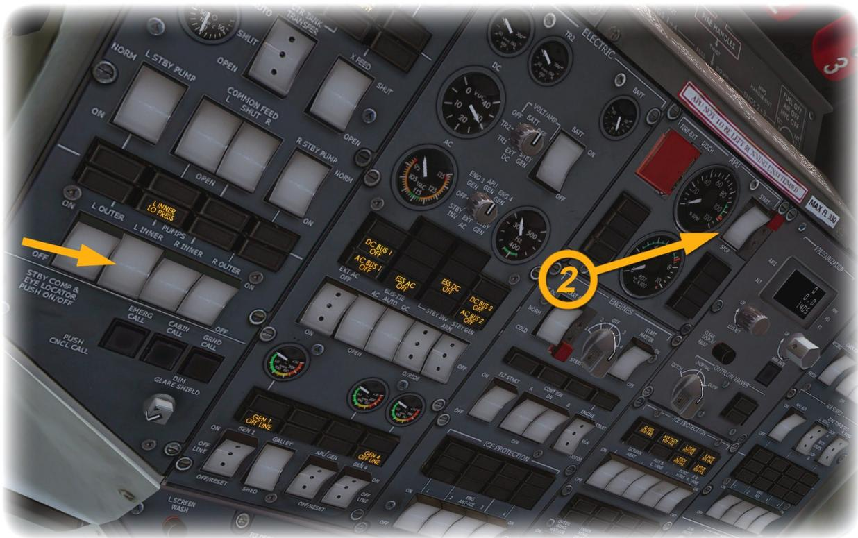
Before you start the APU, make sure you switch on the left inner Fuel Pump in order to provide fuel for the APU.
