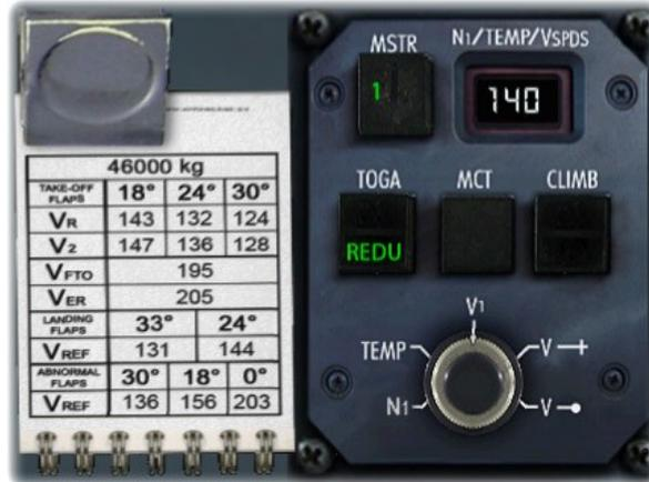
Now select  $V_{CROSS}$  and set the speed to  $V_R$  from the speedcard next to the TRP. The speedcard will always show the correct speeds depending on your aircraft's weight.
