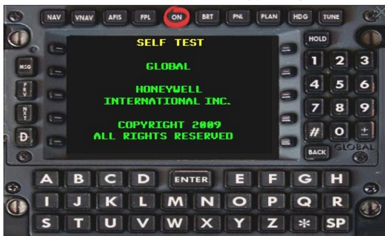
When it is complete, you will be shown the Initialization page. The ICAO code of the nearest airport will be filled in automatically. If it is correct, press the ENTER button.
