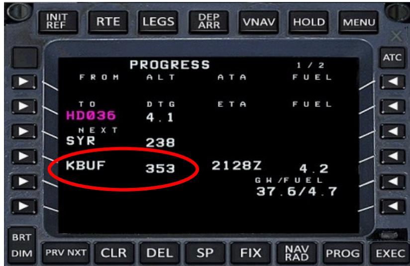
Finally select the LEGS page. Using the FORMAT knob on the EFIS control panel select PLAN. Press LSK 6R to step through and verify on the the map display the proper route. Look at any climb restricted altitudes that are part of the SID. If there a restriction, now would be a good time to set in the the MCP altitude window. In this case the LOGAN6 has no constraints.
