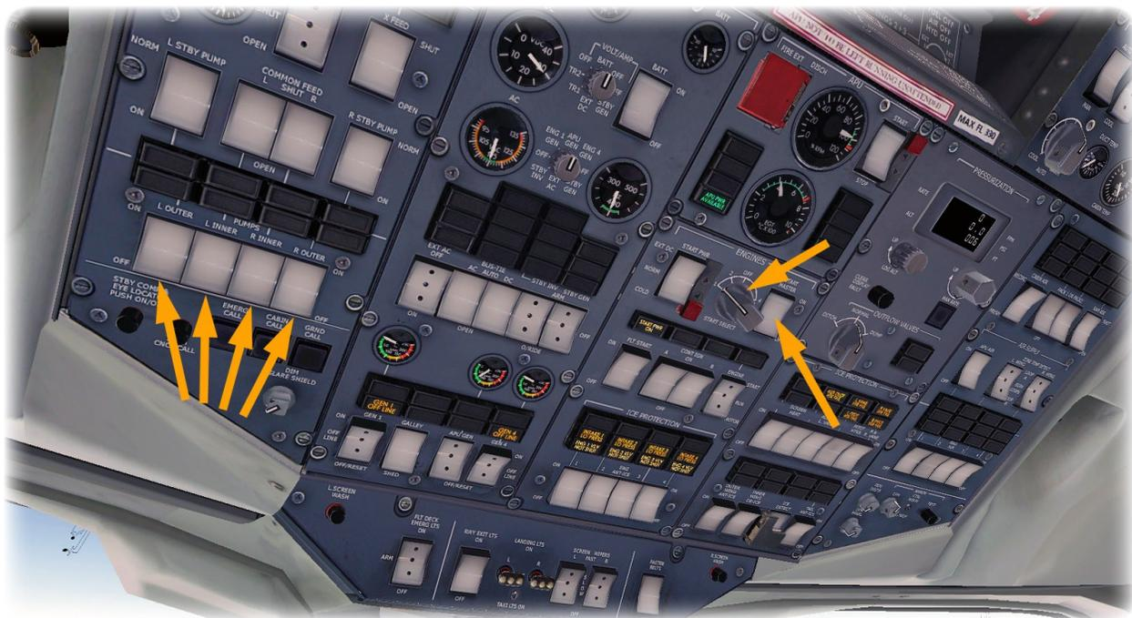
Now to start the engine start motor, click the ENGINE switch. It moves to the START Position and the engine starts to spin.
